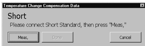
Figure C-26 Temperature Change Compensation Data screen when measuring the short connection
